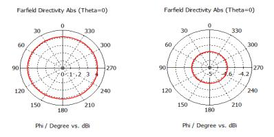
**Fig. 7.** Plot of directivity for theta = 0 for simple patch = 0 for EBG antenna.
