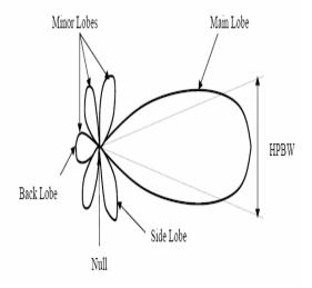
Fig. 3. Radiation pattern of HPBW form.
