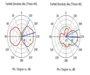
Fig. 8. Plot theta = 90 for antenna, directivity for theta = 90 EBG based antenna.
