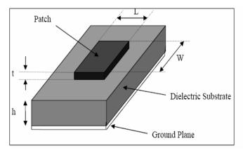
Fig. 4. Microstrip Patch Antenna.
