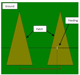
**Fig. 2.** Patch element antenna array.
